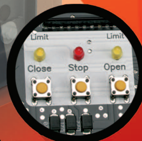
Built-in three push button station
