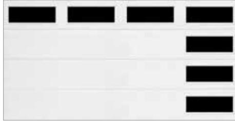
Clear windows may be arranged vertically or horizontally on Colonial, Ranch and Contemporary panels. Windows placed in the bottom section of a door must use DSB 1/8" or tempered glass.
